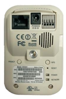
The picture below shows the back of the Wi-Fi camera. The Privacy button is on the left side.
